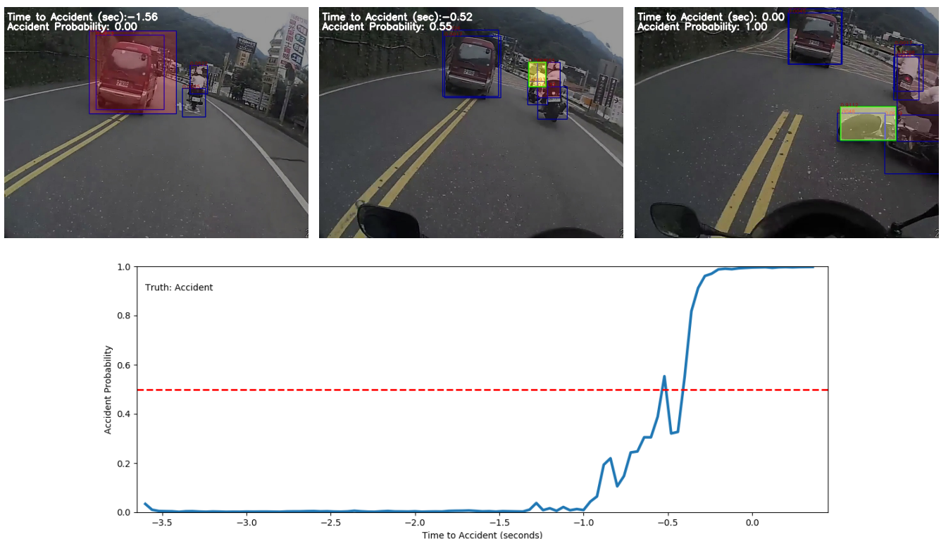
Figure 1: Top row: CNN-predicted Regions of Interest, RoI (in blue) for 3 frames from a traffic video involving an accident at t = 0 second mark. Above each RoI is shown its attention value (in red). Higher the attention, the higher the chance that the corresponding RoI could be involved in an accident. RoIs with attention value above 0.4 are plotted in green boxes. The time to accident and the probability of accident are quoted within each frame. Bottom row: RNN is used to predict showing the probability of accident (along y-axis) at each of the 100 frames (each frame is 0.04 seconds long). RNN triggers an alarm if accident probability goes above the trigger threshold of 50% (red dashed line).
